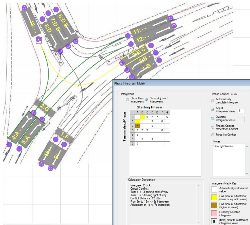
Figure 11 - Manual adjustment of Phase Intergreen
